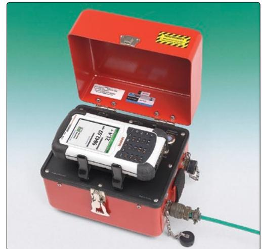
● Model GK-405 Vibrating Wire Readout.
