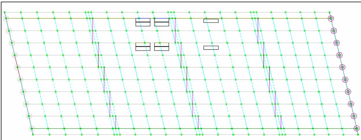
Figure 4 2-D model of Defiance County Hopkins St. Bridge - Span A.
