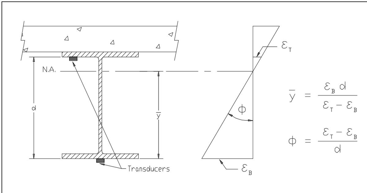
Figure 26 Illustration of Neutral Axis and Curvature Calculations
