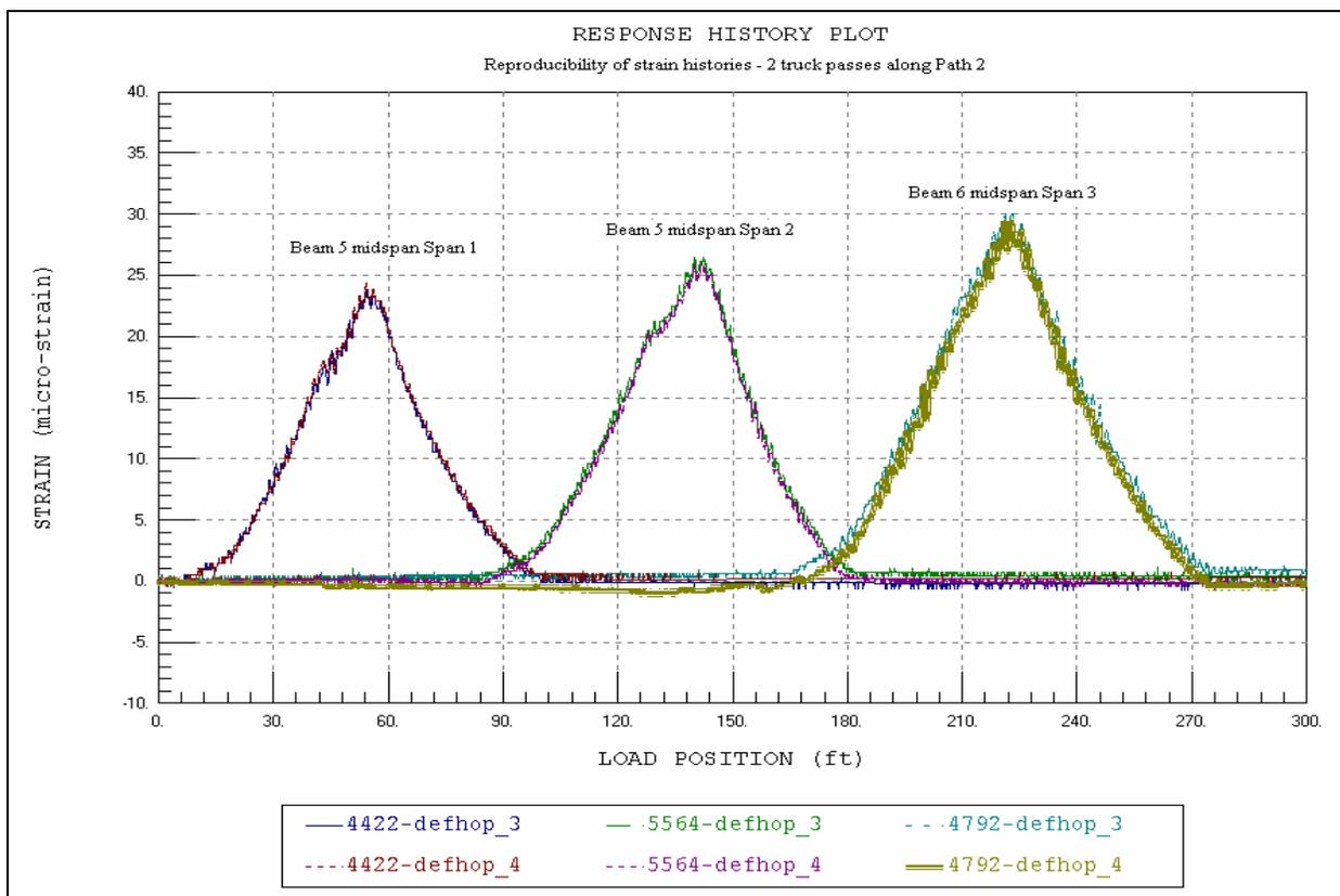
Figure 3 Reproducibility of load test procedures and structural response.
