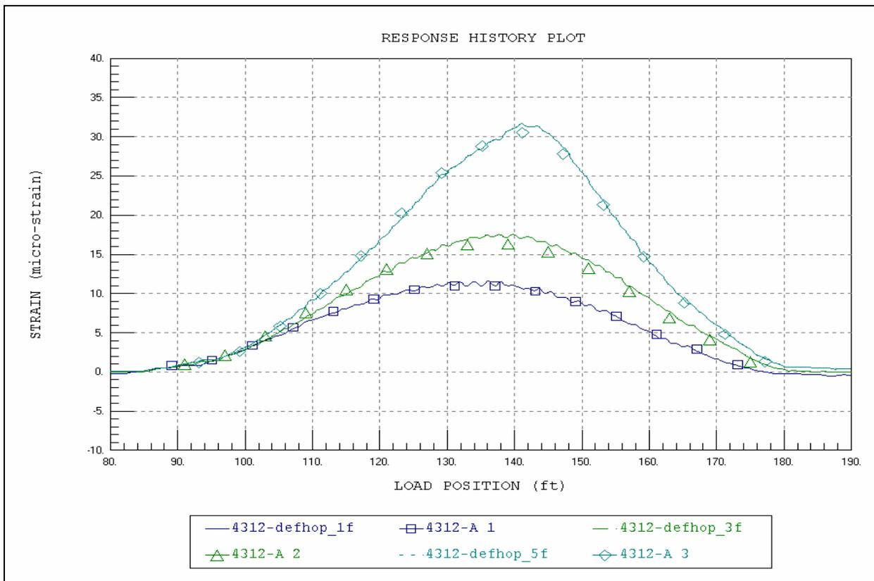
Figure 19 Span B – Beam 11 midspan.
