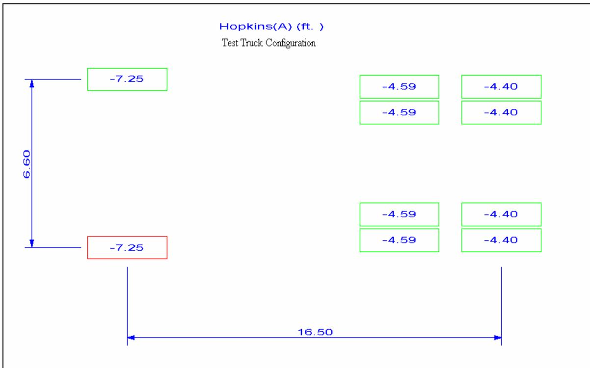
Figure 2 Load Configuration of Test Truck.
