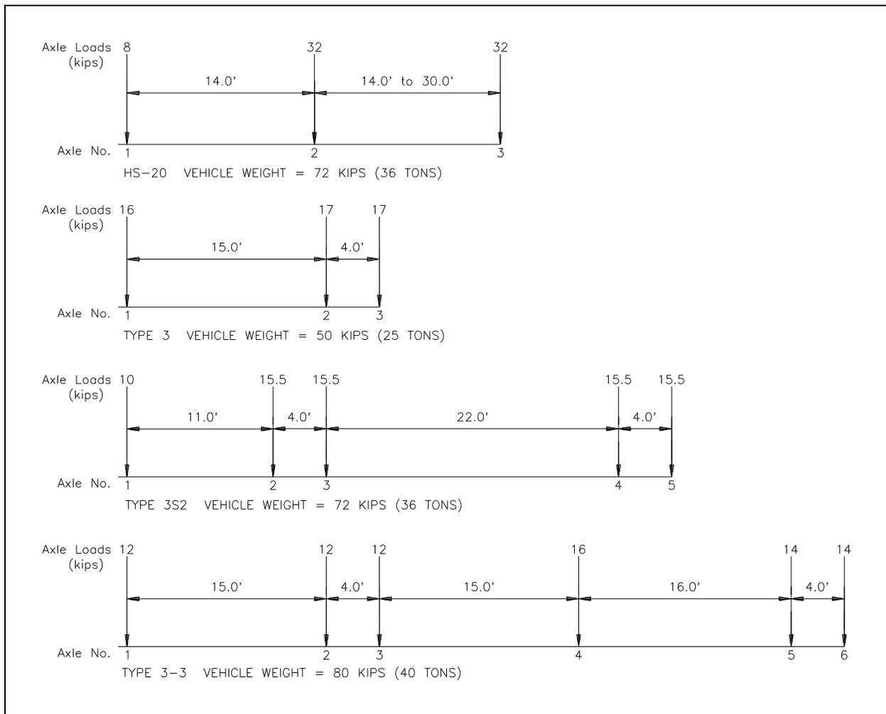
Figure 27 AASHTO rating and posting load configurations.
